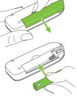
Insert new battery with correct +/- position (Alkaline 1.5 V, type AAA, LR03 or AM4).
